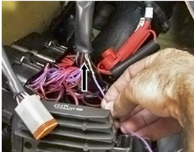
Remove o-ring from end of diagnostic connector.
