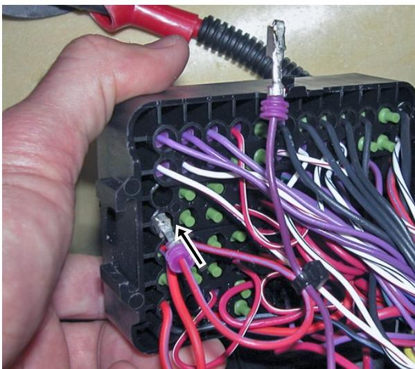
Insert end of purple wire (supplied item #4) into location 'F11'. (Listen for a click!) Pull back on wire to ensure terminal is locked in place.
