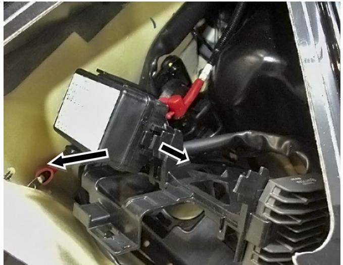
Inside hull flip electrical component support on its side to access voltage regulator. Disconnect black and gray electrical connectors from voltage regulator.
