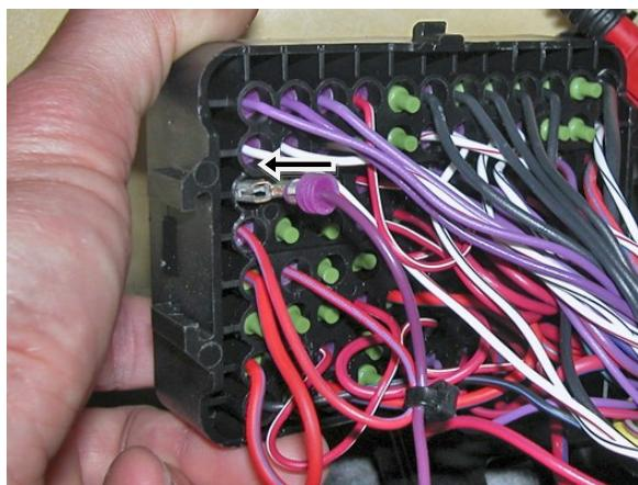
Flip fuse box over to view fuses. Install supplied fuse into fuse panel across locations 'E11 & F11'. Replace bus bar removed previously (row 'D').
