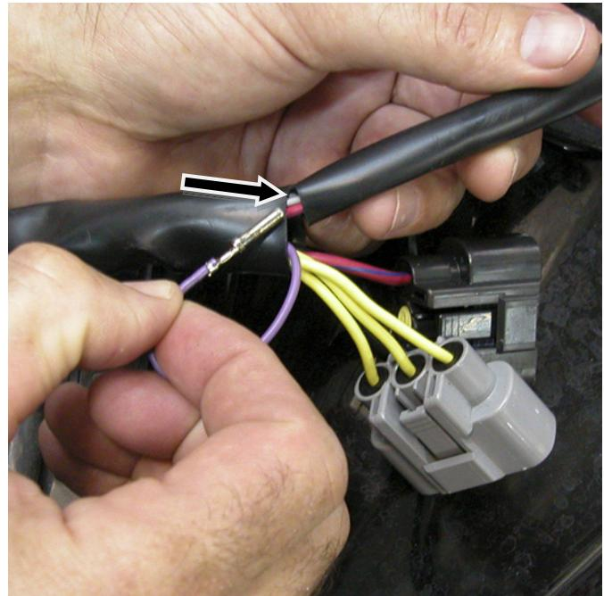
Insert and feed longest end of Electrical Harness Wire (supplied item #4 – purple wire) into end of harness sheath closest to fuse box.
