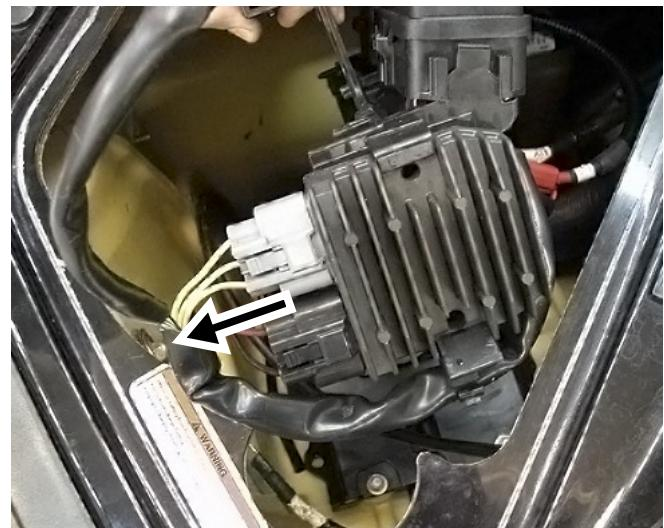
Follow voltage regulator wiring harness from connectors back to fuse boxes.
