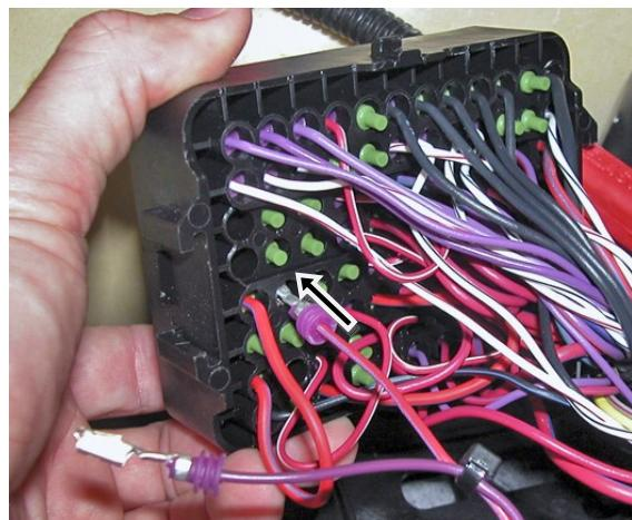
Insert other end of red wire (supplied item #4) into location 'E11'. (Listen for a click!) Pull back on wire to ensure terminal is locked in place.
