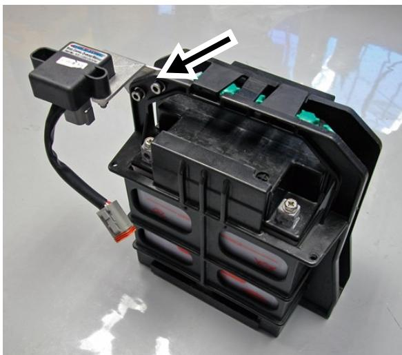
Secure S.C.O.M. bracket to battery holder with supplied hardware (supplied item #2). **NOTE: Do not over tighten bolts.**
